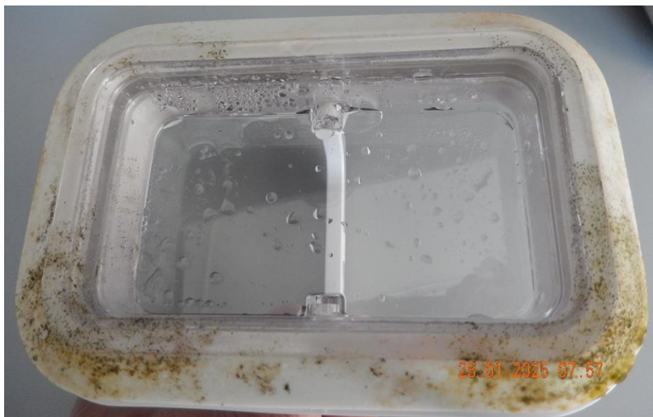
Figure 12. Interior appearance of the container lid, showing shapes adhered to the polyethylene, especially on the illuminated side. The rest of the surface is remarkably clean
