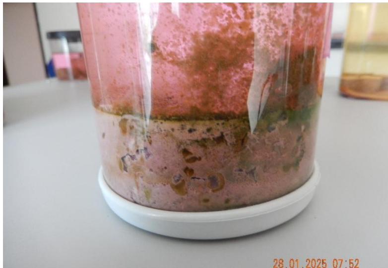
Figure 17. Appearance of organic carbon formations within a cylindrical polyethylene container, containing water, QBLOCKS™ and Pumice soil
