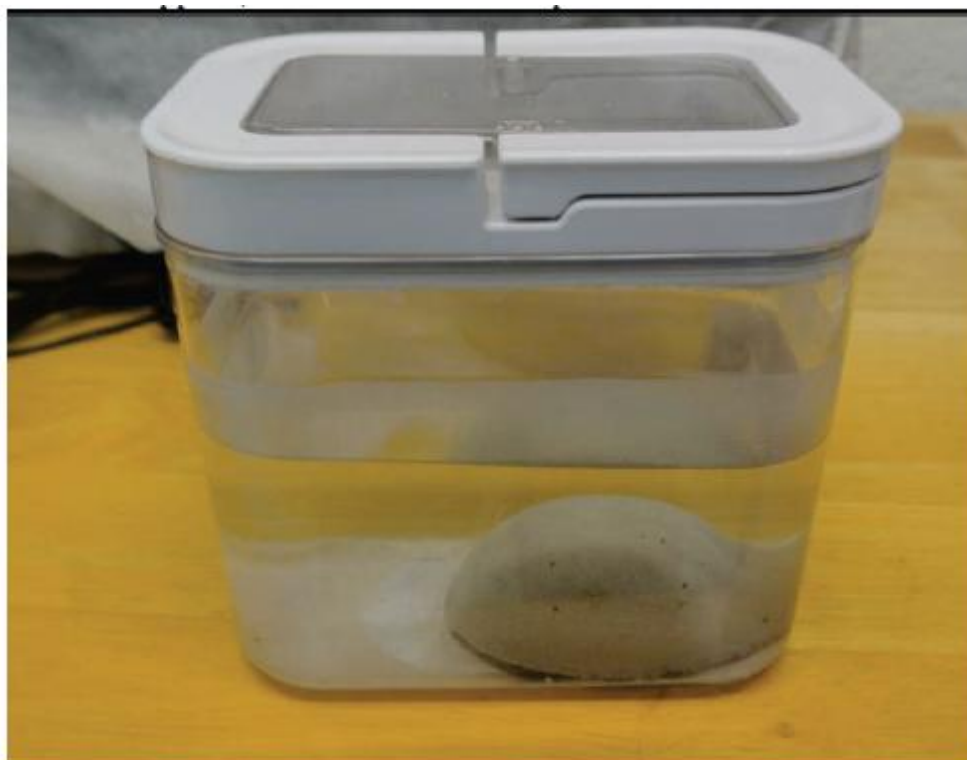
Figure 4. In a relatively airtight plastic container, a 100-gram QBLOCK TM was placed in 400 ml of distilled water. (June 2022)
