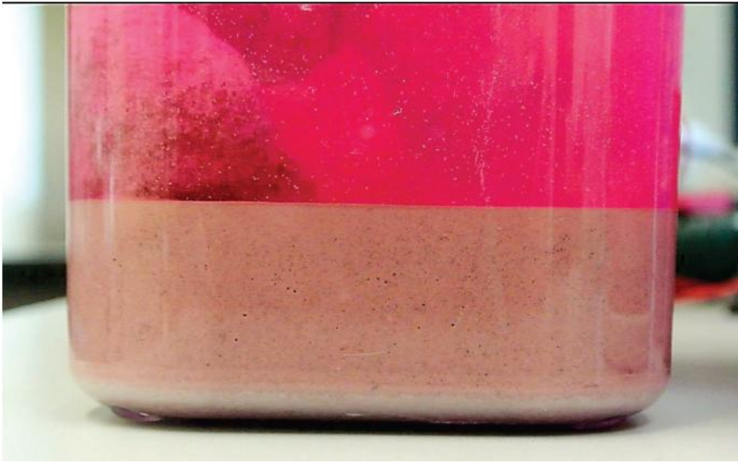
Figure 5. The photograph shows the initial appearance of the plastic container, once the stone and pumice soil were added. Pumice stone tends to float when dissolved oxygen levels are elevated
