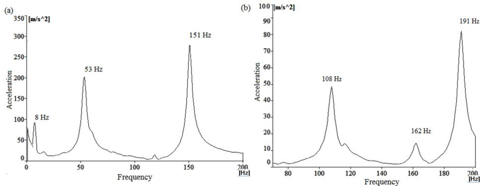
Figure 8. Frequency response of a) beam without absorber b) beam with absorbers when absorbers tuned to impose node at  $0.4L$  and  $0.6L$ , by experimental modal analysis
