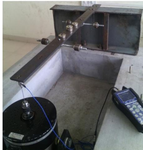
Figure 5. Experimental test on cantilever beam supporting lumped masses with two absorbers tuned to impose nodes
