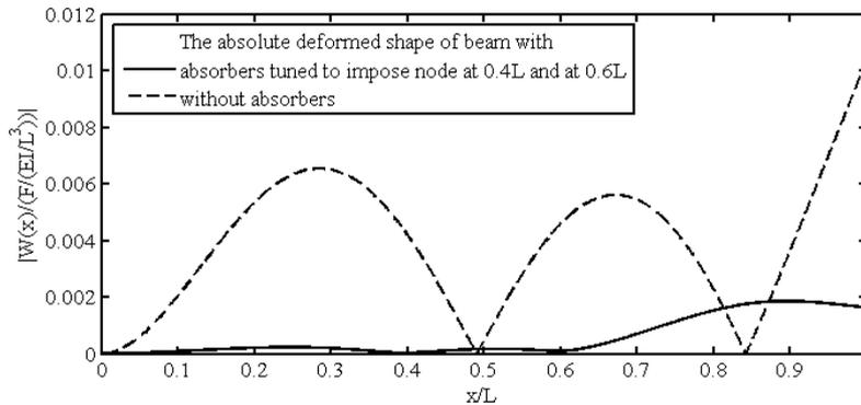
Figure 3. The absolute steady-state response of beam with and without absorbers to impose nodes at  $0.4L$  and  $0.6L$ , for the absorber parameters listed in Table 1
