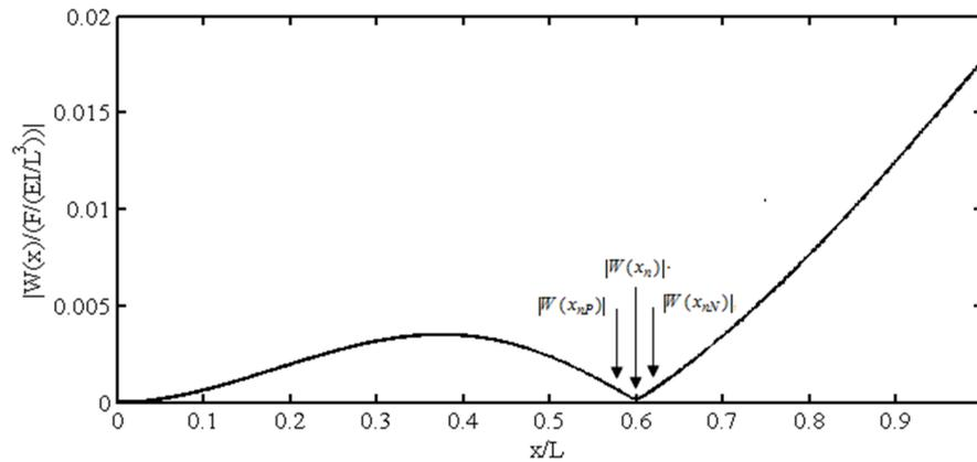
Figure 2. Illustration of condition  $|W(x_n)| < |W(x_{nP})|$  and  $|W(x_n)| < |W(x_{nN})|$ , used to find frequency of absorber
