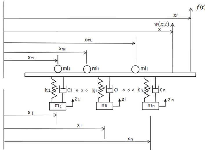
Figure 1. Beam with variable stiffness damped multiple absorbers subjected to localized harmonic excitations
