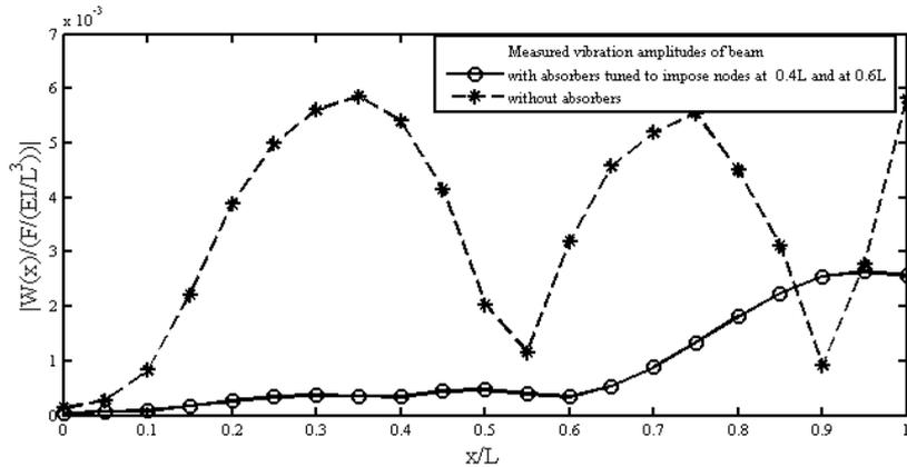
Figure 6. Measured vibration amplitude of beam with absorber tuned to impose nodes at  $0.4L$  and  $0.6L$  and without absorber
