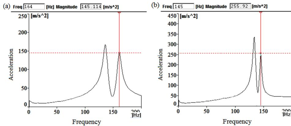
Figure 7. Frequency response of a) absorbers attached at  $0.3L$  b) absorbers attached at  $0.65L$ , by experimental modal analysis when absorbers tuned to impose node at  $0.4L$  and  $0.6L$
