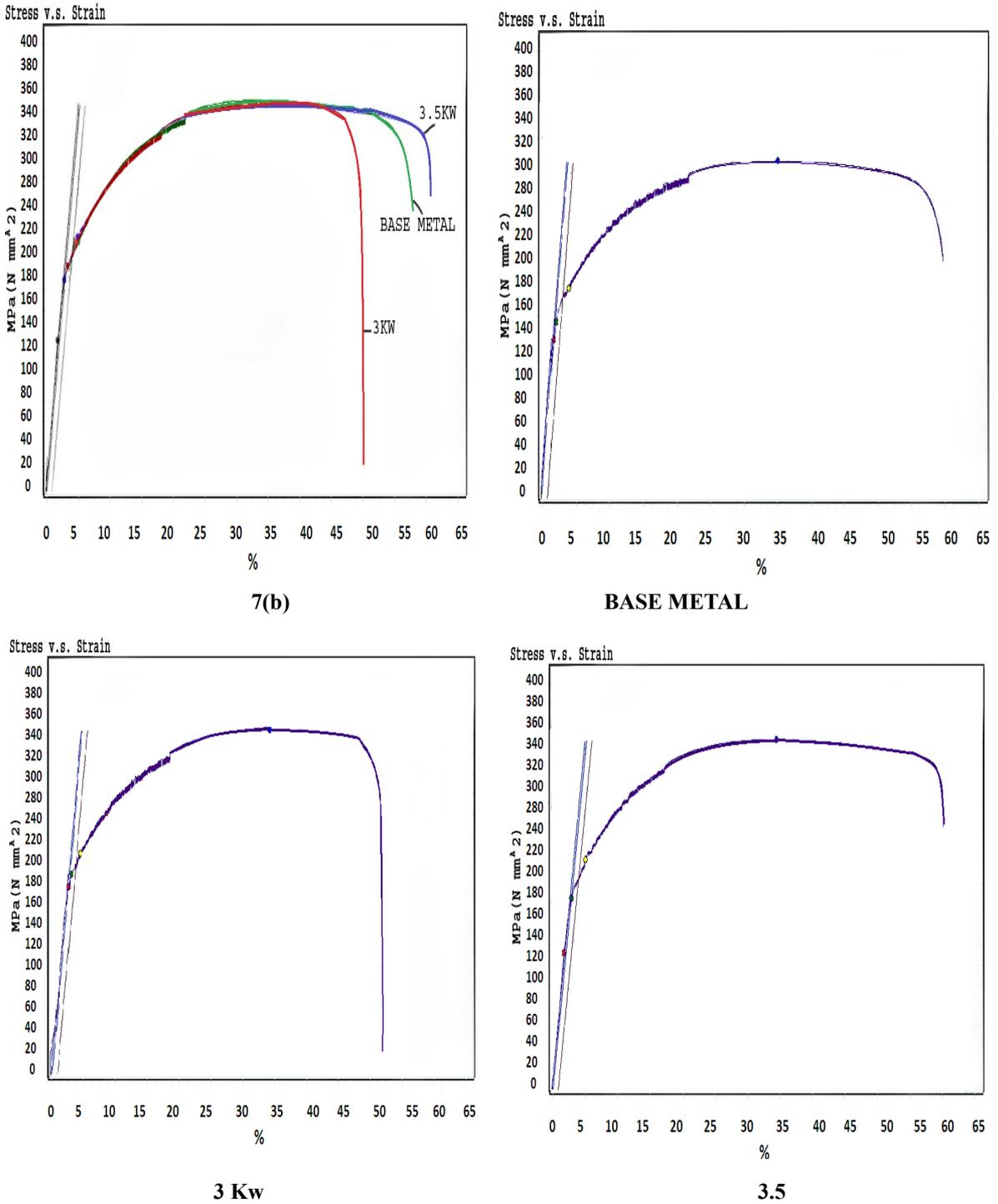
Figure 7(b). Comparison of the stress-strain curves of high temperature tension tested 316L(N) base metal, 3.0KW laser welded and 3.5Kw laser 316L(N) weldments showing serrated yielding
