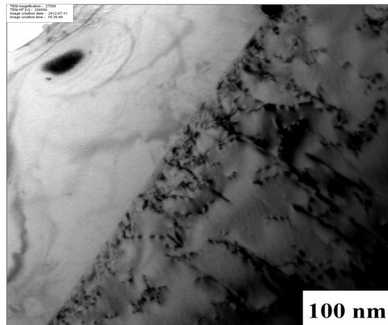
Figure 4. Bright field TEM microstructure of the grain boundary region showing carbonitrides on dislocations
