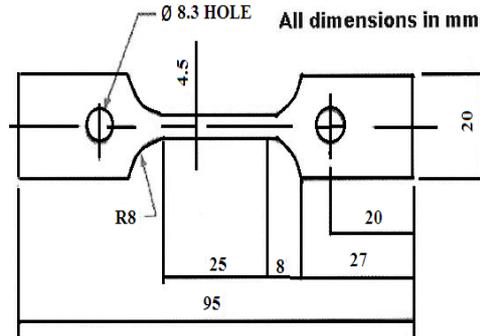
Figure 1. Tension test sample design
