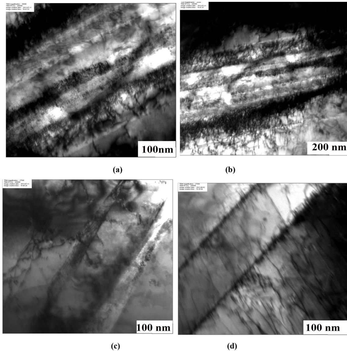
Figure 3. (a) Bright field TEM microstructure showing high density of dislocation and deformation bands; (b) Bright field TEM microstructure showing deformation bands and dislocations; (c) Bright field TEM microstructure showing deformation bands and Dislocations; (d) Bright field TEM microstructure showing high density of dislocation
