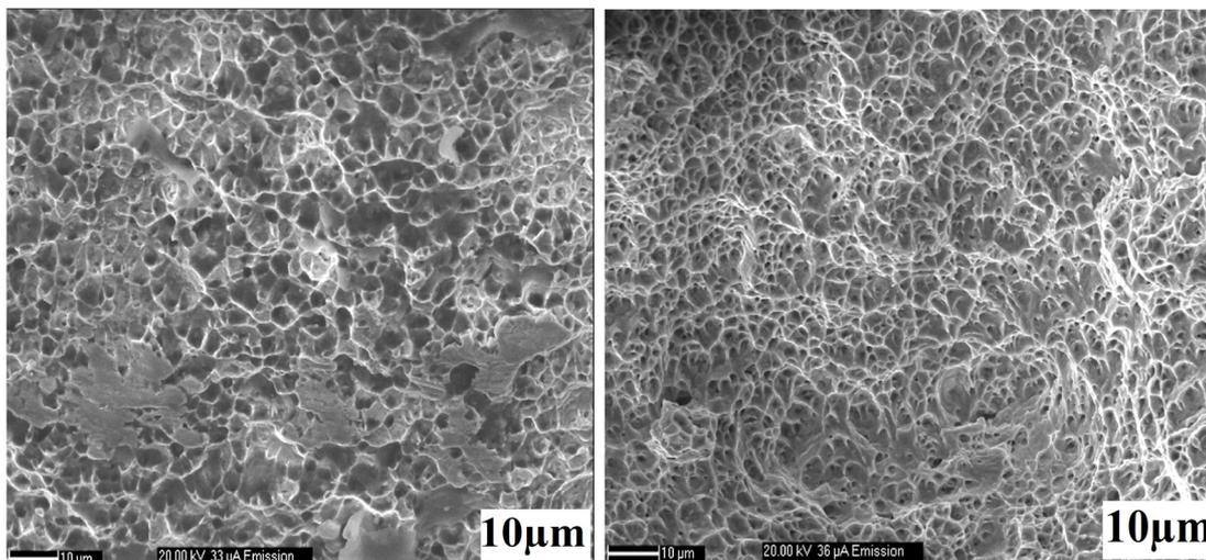
Figure 5. (a) SEM microstructure of the room temperature tension tested 3.0 KW laser welded 316L(N)SS; (b) SEM microstructure of the room temperature tension tested 3.5KW laser welded 316L(N)SS
