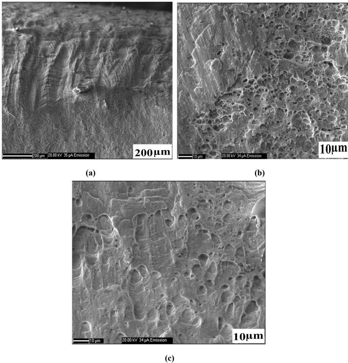
Figure 6. (a) SEM microstructure of the high temperature tension tested 3.0 KW laser welded 316L(N)SS; SEM microstructure of the high temperature tension tested 3.0 KW laser welded 316L(N)SS; (c) SEM microstructure of the high temperature tension tested 3.5 KW laser welded 316L(N)SS
