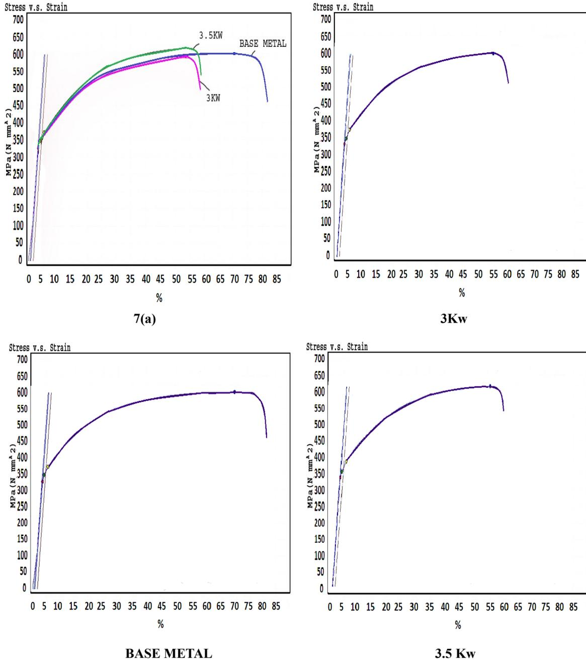
Figure 7(a). Comparison of the stress-strain curves of room temperature tension tested 316L(N) base metal, 3.0 KW laser welded and 3.5 Kw laser 316L(N) weldments
