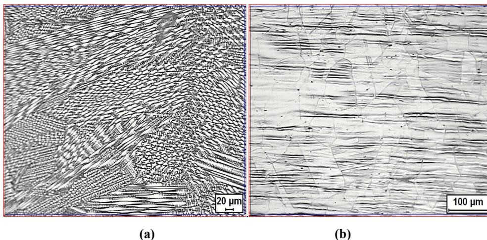
Figure 2. (a) Optical microstructure of the 3.5KW laser welded fusion zone; (b) Optical microstructure of the 316L(N) basemetal
