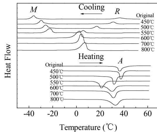
Figure 3. The DSC curves of the Ni-50.5a.t.%-Ti super-elastic wire annealed with different annealing temperatures (annealing temperature: 550°C, cold-drawing amount: 39%)
