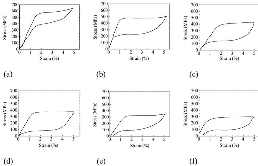
Figure 5. The hysteresis loop of the samples with the annealing temperature of (a) 450, (b) 500, (c) 550, (d) 600, (e) 700, and (f) 800 (39% cold drawing, annealing for 20min)
