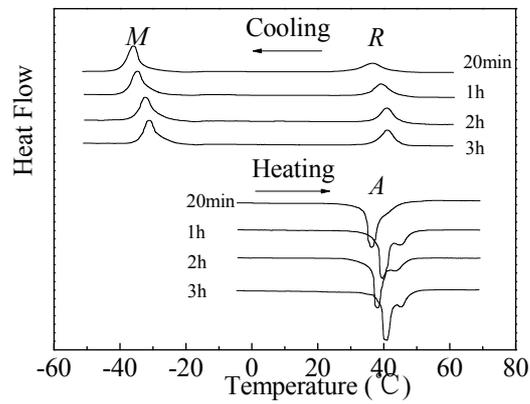
Figure 1. The DSC curves of the Ni-50.5a.t.%-Ti super-elastic wire annealed with different temperatures (annealing time: 20min, cold-drawing amount: 39%)
