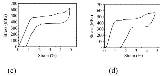
Figure 6. The hysteresis loop of the samples with the annealing time of (a) 20min, (b) 1h, (c) 2h, and (d) 3h (39% cold drawing, annealing at 450 °C)
