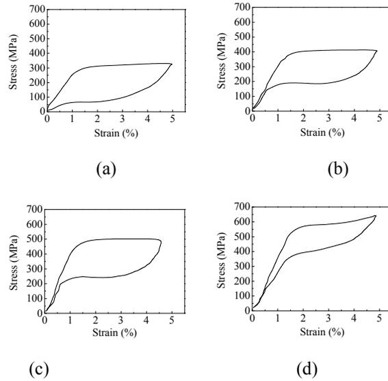
Figure 4. The hysteresis loop of the samples with the cold drawing amount of (a) 6.9%, (b) 22%, (c) 31%, and (d) 39% (annealing at 450 °C, for 20min)
