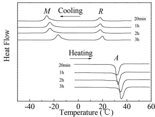
Figure 2. The DSC curves of the Ni-50.5a.t.%-Ti super-elastic wire annealed with different annealing times (annealing temperature: 450°C, cold-drawing amount: 39%)
