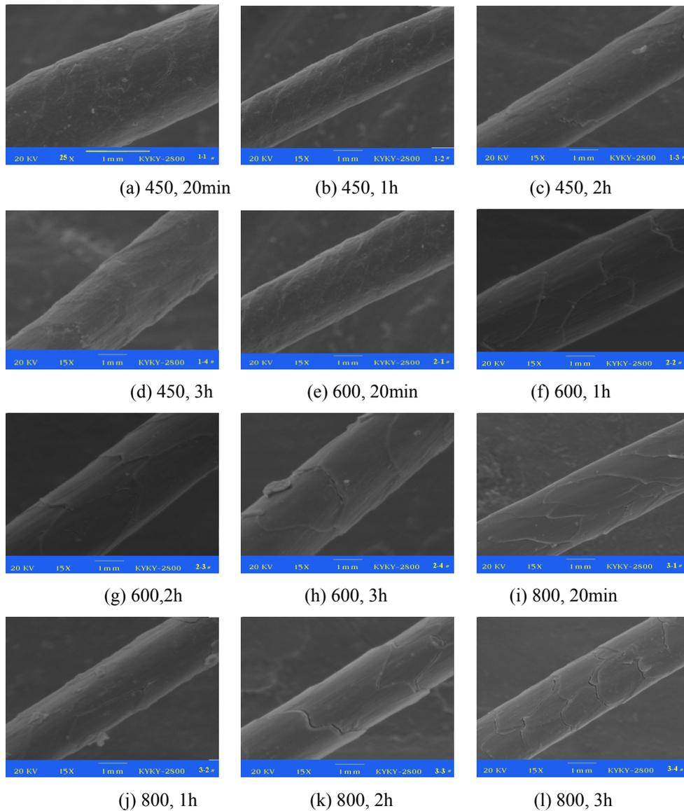
Figure 7. The surface morphology of Ni-Ti alloy wire after the second mass of annealing (39% cold drawing)
