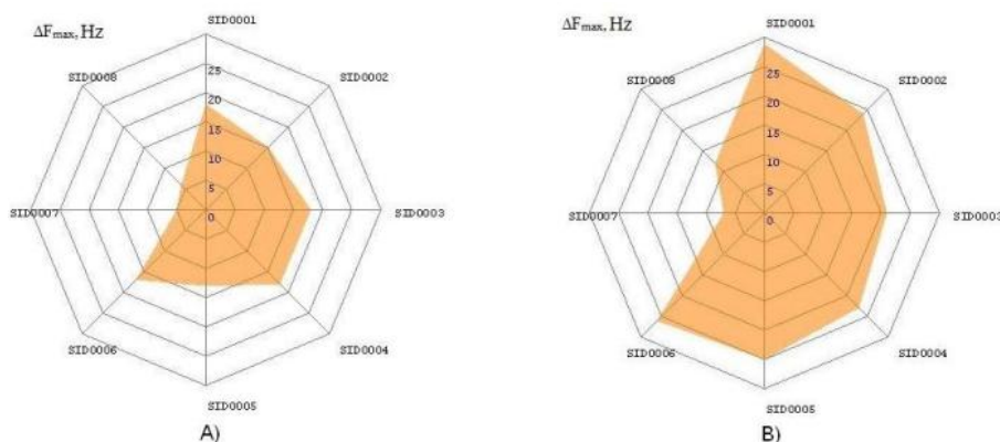
Figure 3. "Visual imprints" of the maximum sensor signals in the EGP over the injected chicken leg quarters. (A) Basic formulation, (B) modified formulation. Axes are indicated by sensors in the matrix
