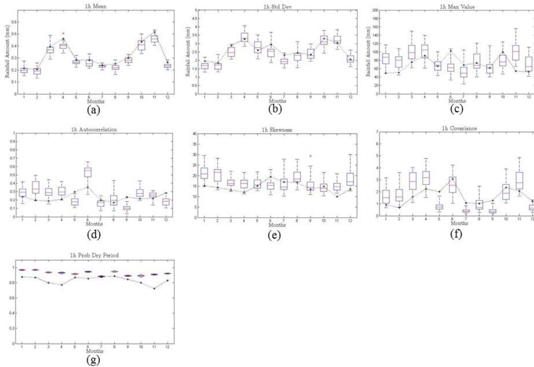
Figure 3(a-g). Comparison of statistical characteristics between simulated hourly series (box plots) and observed series (dotted line) for station Ampang, Selangor (2001-2010)
