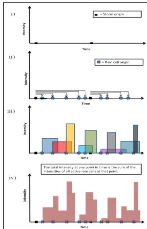
Figure 1. Schematic diagram of the Neyman-Scott model
