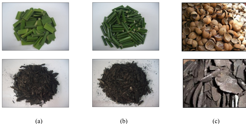
Figure 4. Biochar preparation from (a) Typha, (b) Cyperus, and (c) coconut shells after burning their air-dry weight by using Muffle Furnace at 400-500 °C
