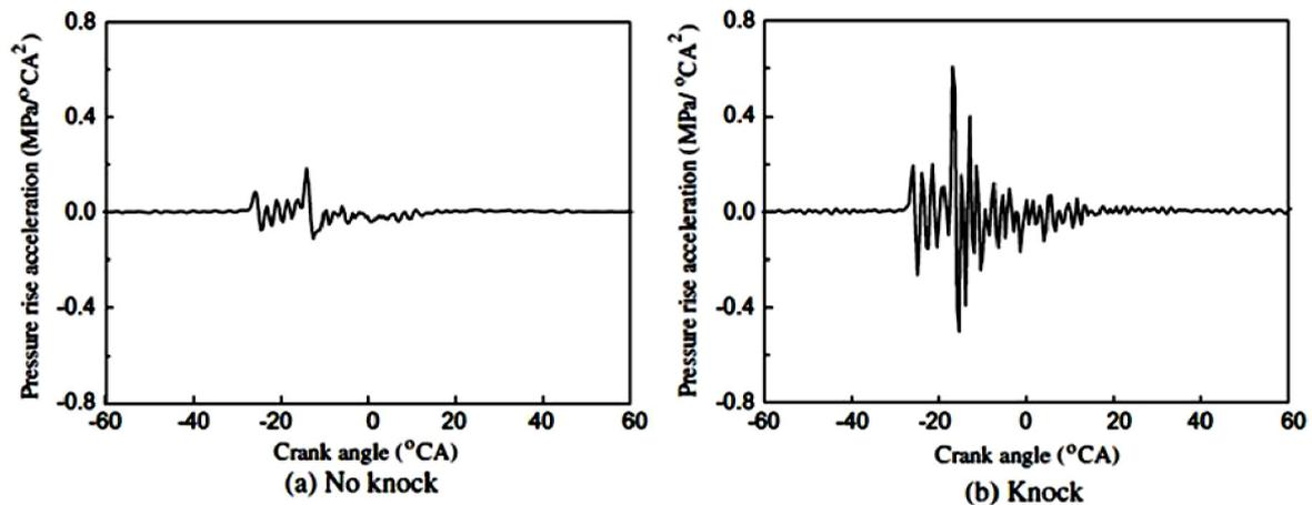
Figure 3. Patterns of normal vibrations (no-knock) and detonation (knock) (Hou et. al., 2009)
