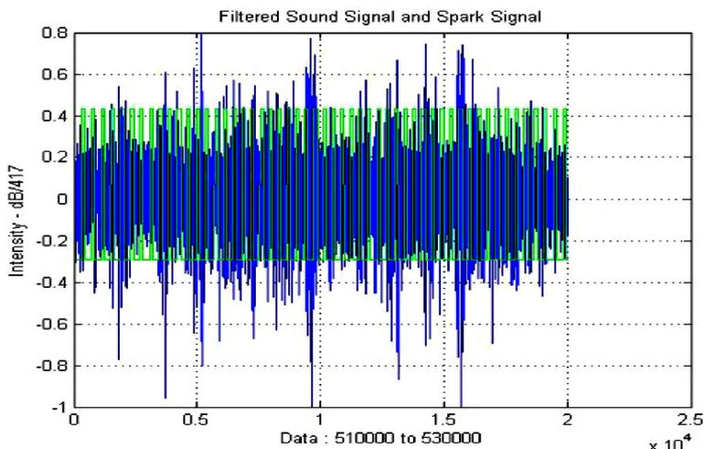
Figure 8. A recorded engine sound signal in normal conditions that has been filtered
