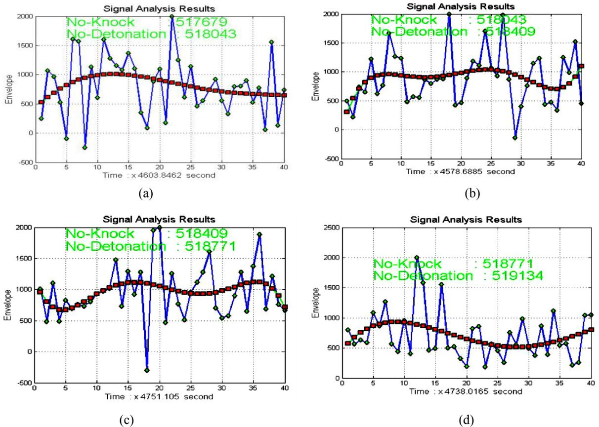
Figure 12. The envelope function and regression, a) cycle 1, b) cycle 2, c) Cycle 3, d) cycle 4, for the engine noise signal in abnormal conditions (no-knock)
