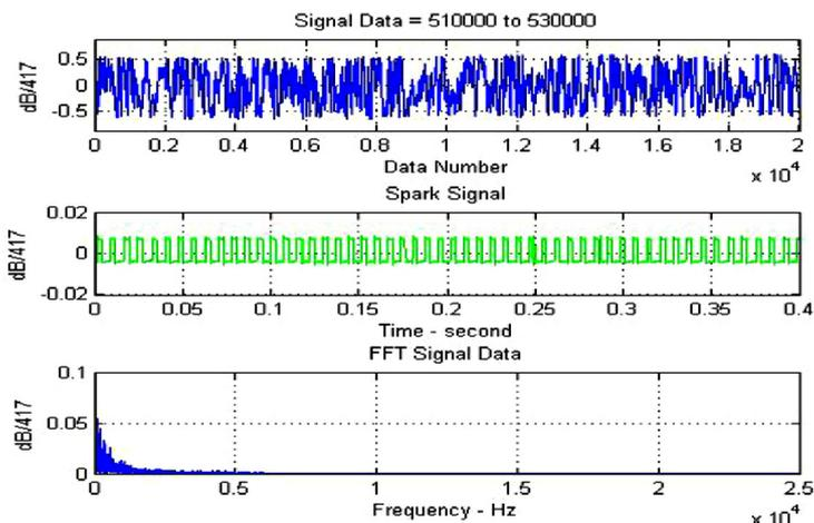
Figure 7. A recorded engine sound signal in normal conditions and its FFT
