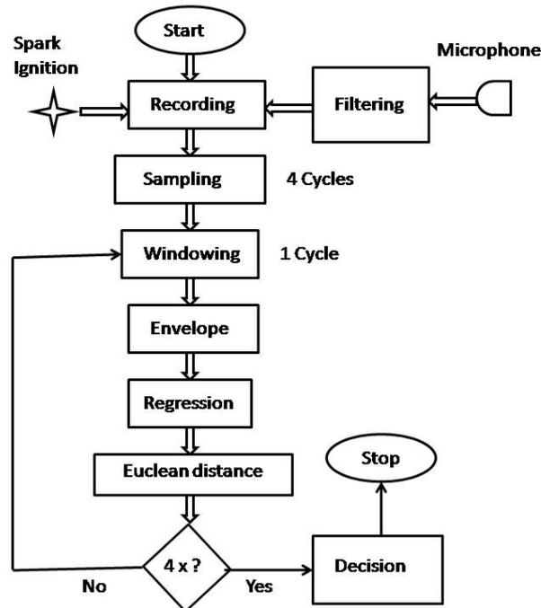
Figure 5. Data processing of detonation sound vibration patterns
