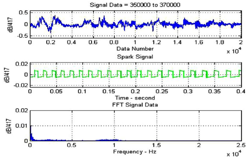
Figure 9. A recorded engine sound signal in detonation conditions and its FFT
