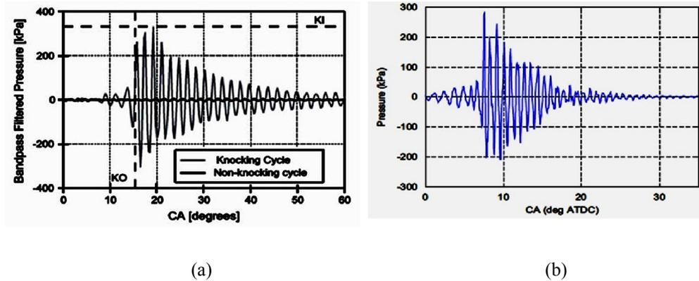
Figure 2. Shape of a detonation vibration pattern (knock): (a) Rothamer et.all (2012), (b) Galloni (2012)
