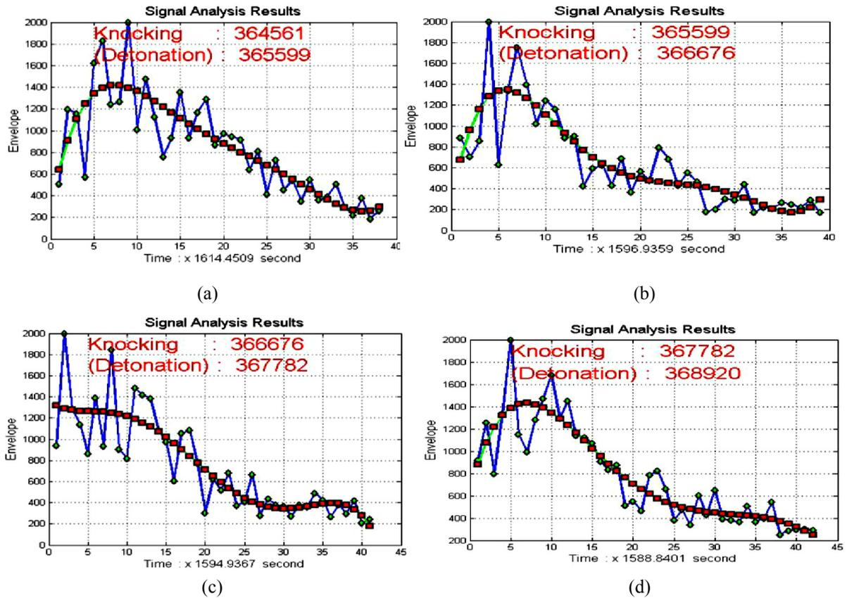
Figure 13. The envelope function and regression, a) cycle 1, b) cycle 2, c) cycle 3, d) cycle 4, engine noise signal in the condition of detonation (knocking)
