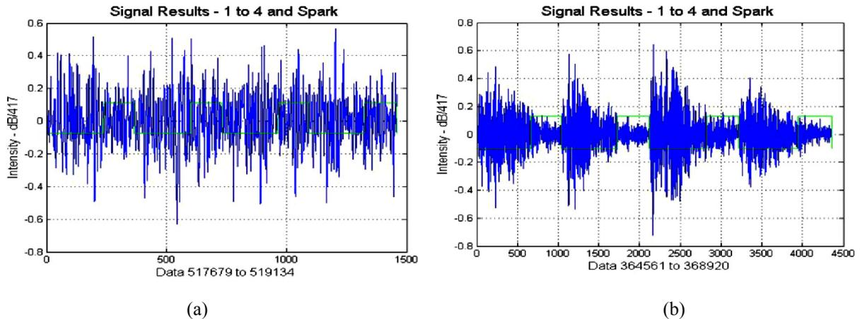
Figure 11. Taking the signal sample for a 4 cycles ignition for engine in: (a) normal engine (no-knock), (b) detonation conditions (knock)
