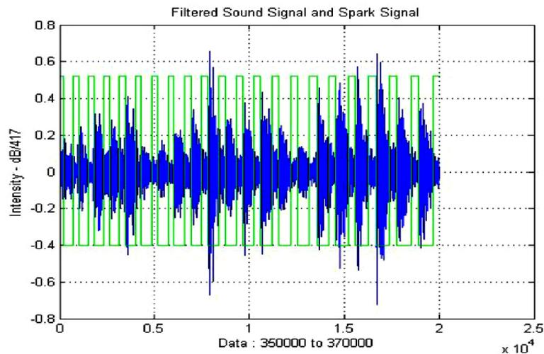
Figure 10. A recorded engine sound signal in detonation conditions that has been filtered
