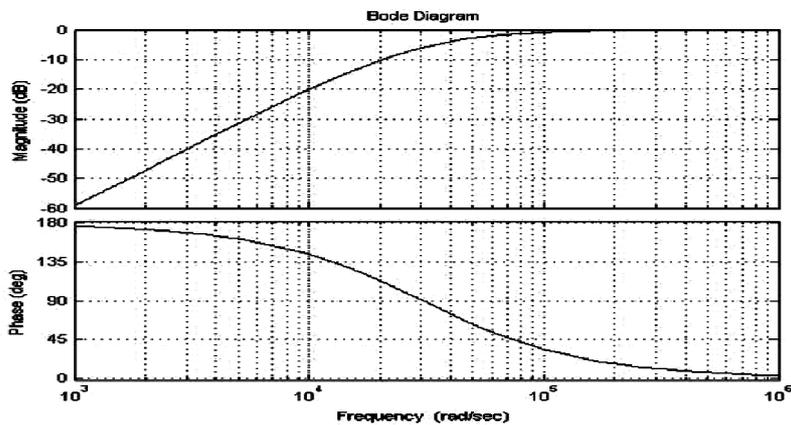
Figure 6. A Bode-plot analysis for the Sallen-Key HPF
