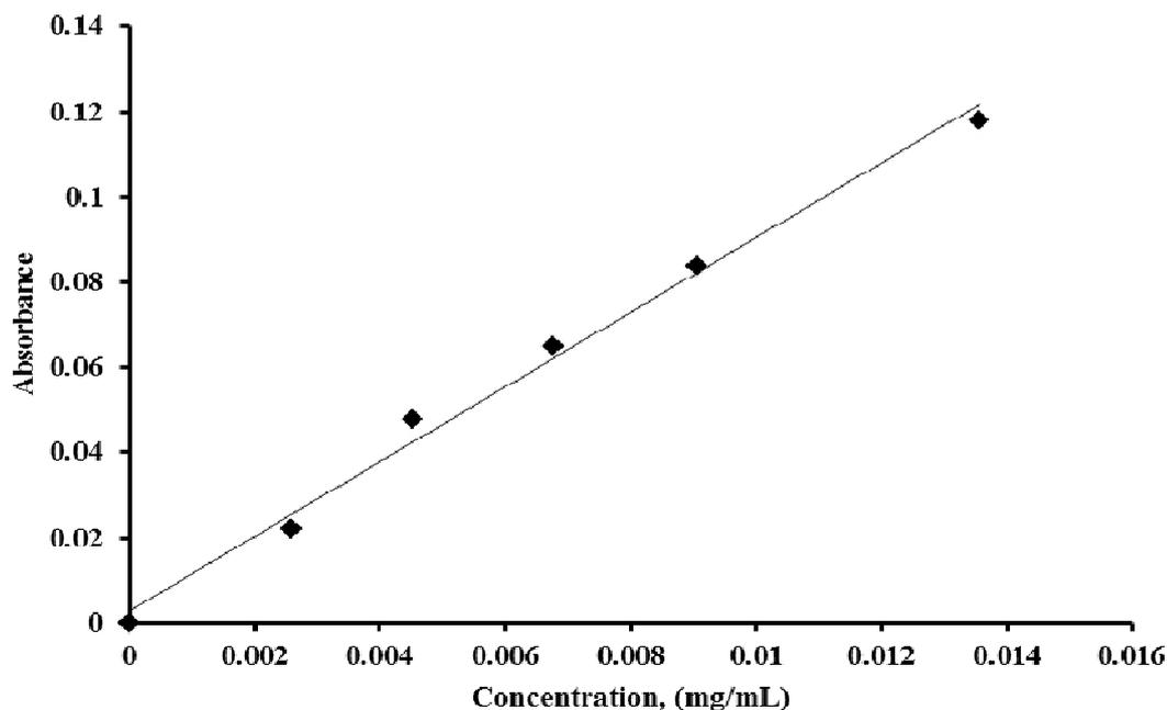
Figure 5. Calibration curve for protein determination using the Lowry Protein Assay at 650 nm; concentration of standards ranged from 0-0.014 mg/mL;  $R^2 = 0.9916$
