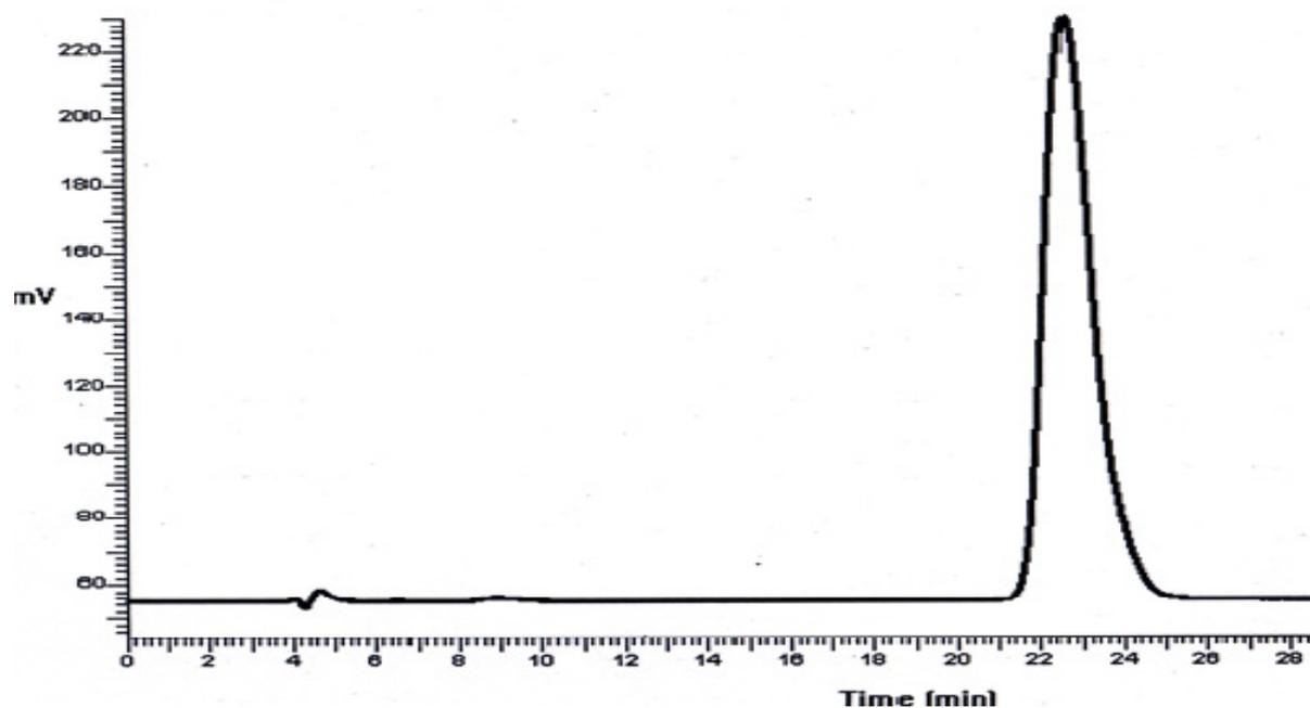
Figure 2. HPLC of genistein standard (100 ppm); retention time is 22.7 minutes
