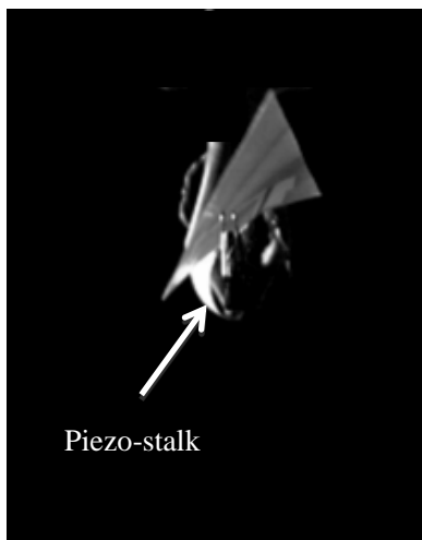
Figure 19. Image at 8.0m/s. Clamping strip interfering flapper motion
