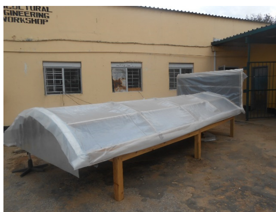
Figure 1. Natural Convection Solar Tunnel Dryer
