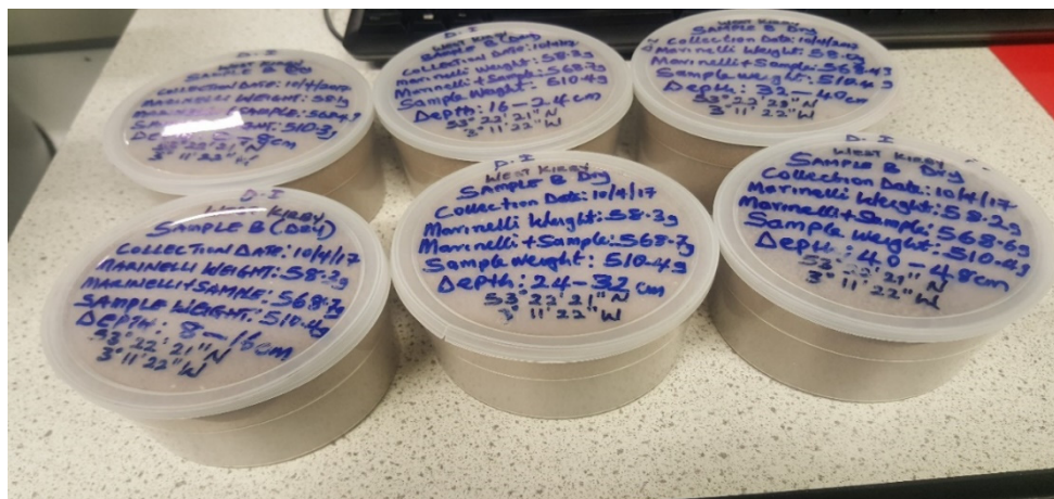
Figure 1. Soil samples in 500ml Marinelli beaker
