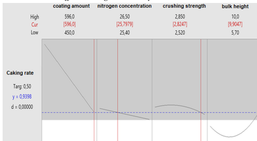
Figure 3. Examination of the effect of parameter values in operating conditions on the caking ratio by regression analysis
