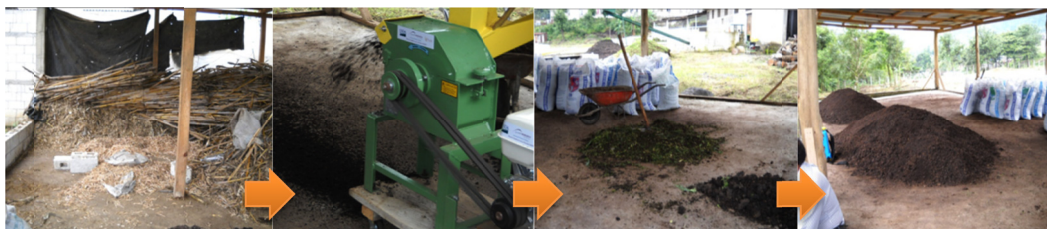
Figure 1. Compost process: Collection of raw material, grinding, mixing and package
