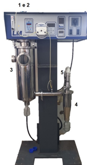
Figure 2. Spray dryer used for drying the Jambu extract, where: (1 and 2) indicate the position of the atomizing nozzle and the air and solution inlets; (3) denotes the drying chamber location; (4) refers to the cyclone; (5) represents the air and fine particle exhaust (non-collected)
