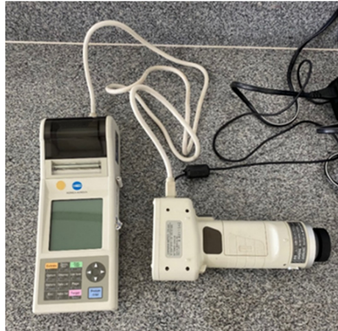
Figure 3. Konica Minolta CR-400 colorimeter
