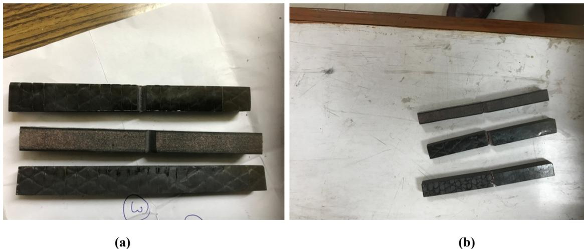
Figure 10. Sandwich composite specimens fractured under Charpy Impact Test
