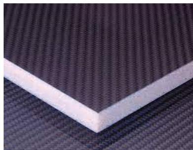
Figure 1. CFRP-Foam-CFRP Sandwich (250x200 mm) Composite
