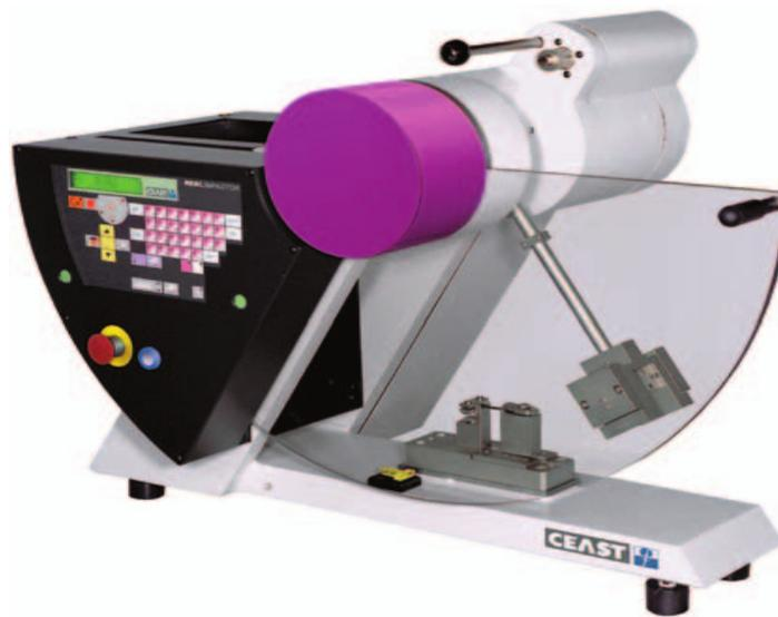
Figure 4. Photograph of Izod and Charpy Impact Tests on Resil Impactor Instrument
