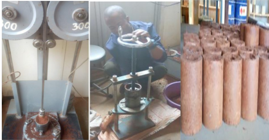
Figure 1. Making compressed stabilized cylindrical blocks
