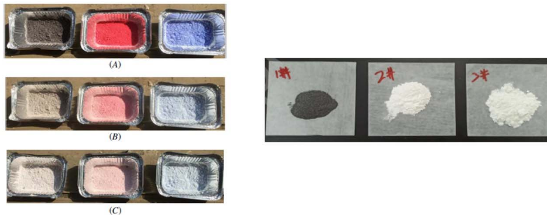
Figure 8. Illustration of the thermochromic powders and Phase Change Materials
