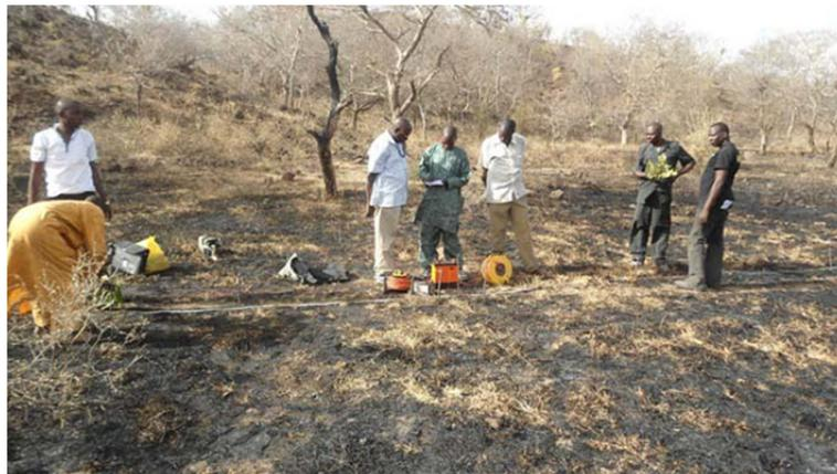
Plate 1. Vertical Electrical Sounding in Kumba crater
