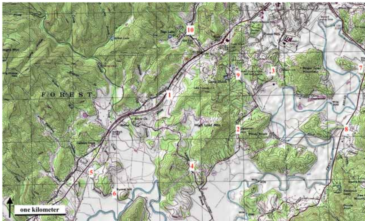
Figure 4. Modified topographic map from the USGS National Map website showing southeast-oriented barbed tributaries flowing to the northeast-oriented French Broad River. Note how the highway and railroad make use of a through (dry) valley. Red numbers identify valleys in the diverging and converging valley complex. The contour interval is 40 feet (13 meters)
