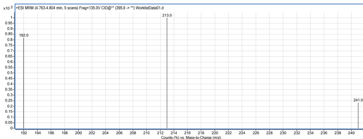
Figure 2. Mass spectroscopy figure of rotenone
