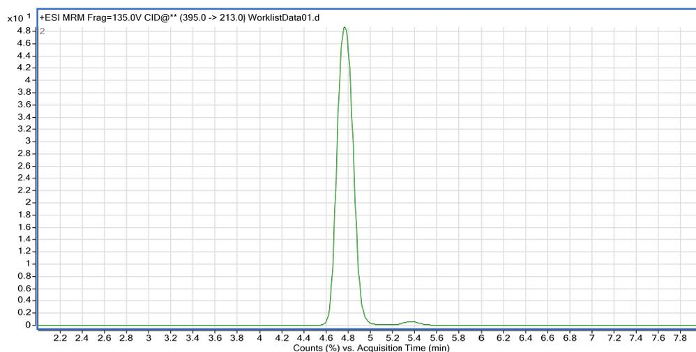
Figure 1. Selected ionization chromatography of rotenone by MRM mode ( $m/z$  395/213)
