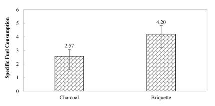
Figure 5. Specific fuel consumption for charcoal and briquette
