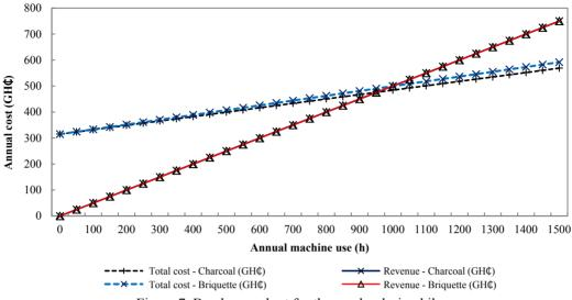
Figure 7 illustrates the breakeven chart for the smoke-drying kiln using charcoal or briquette fuel material.
