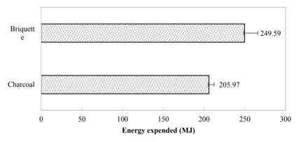
Figure 6. Energy expended by charcoal and briquette fuel materials
