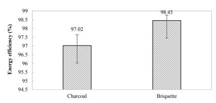
Figure 4. Energy efficiency of the kiln for charcoal and briquette
