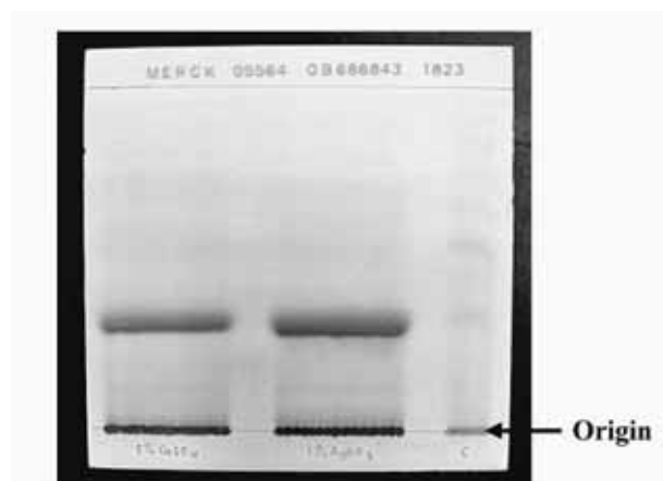
Figure 2. Chromatogram of lettuce extracts after elicited with (a) 5% of \text{CuSO}_4 (w/v) and (b) 1% \text{AgNO}_3 and sprayed with reagent 2,4-dinitrophenylhydrazine (2,4-DNPH).
