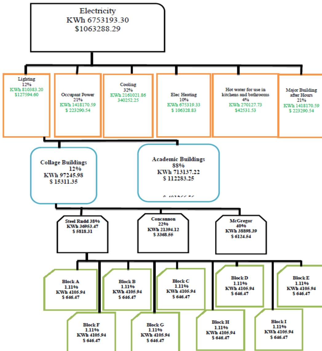
Figure 11. Estimating electricity consumption USQ from January to end of June 2013
