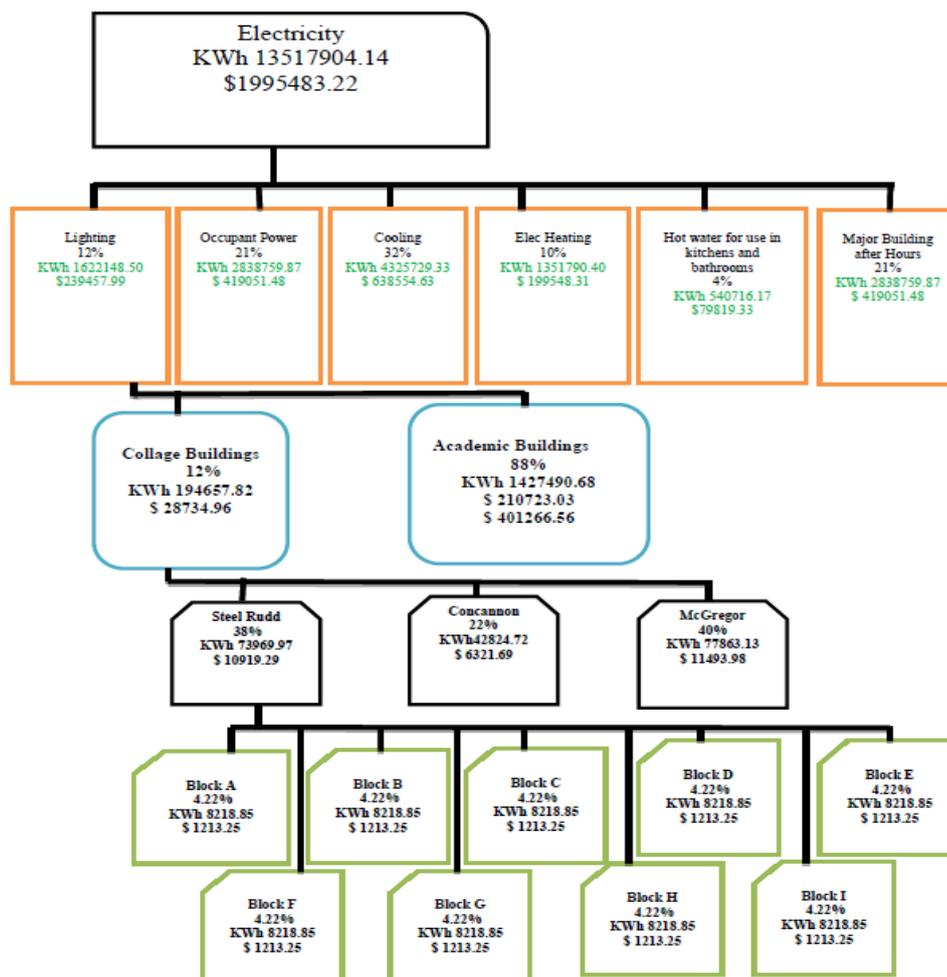
Figure 10. Estimating electricity consumption USQ for 2009
