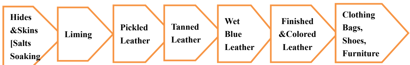
Figure 1. Presents a flow diagram of a tanning-process
