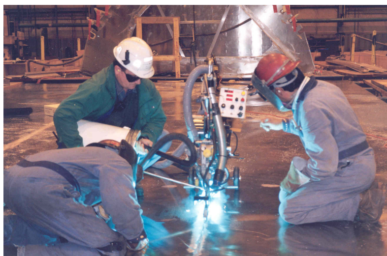
Figure 2. Collecting the welding plume for use in testing instrument response. The black hose connecting to the vacuum cleaner creates a vacuum inside the pail. Note: This photo shows a highly inappropriate practice not to be imitated, namely failure to protect the skin of the face and the hands against exposure to UV emissions from the arc
