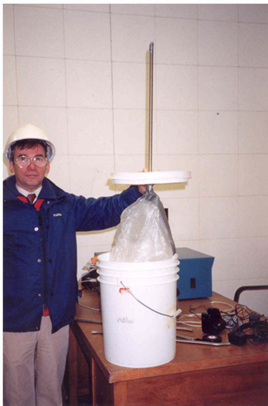
Figure 1. Components of the sampling train. The welding plume flows through the metal tube into the plastic bag when the vacuum cleaner removes the air from inside the pail
