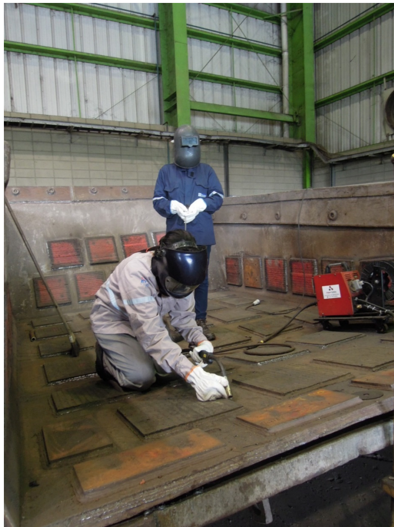
Figure 3. Mock-up showing the welder and the sample-taker. In this test, sampling occurred only during production of the welding plume. Prior testing in the absence of welding confirmed the ability to minimize interference with rapid movement of the welder to avoid hazardous conditions
