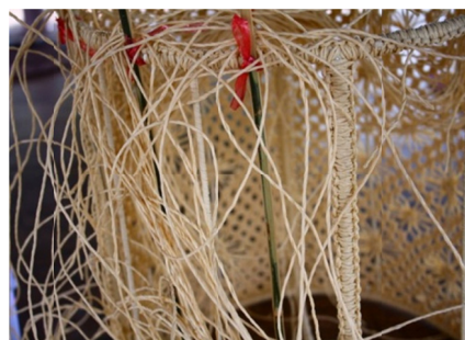
Figure 3. Twine rope around the frame's metal pieces and make weaves in the designed patterns
