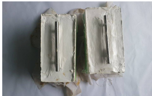
Figure 5. Press the upper mold onto the lower mold with pulp spread inside to produce packaging
