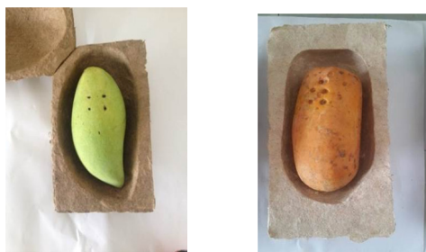
Figure 13. Packaging made from heliconia pulp mixed with cassia leaves extract water
