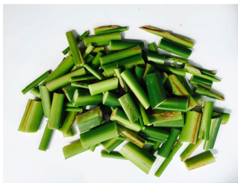
Figure 3. Heliconia stem pieces for refining and boiling to prepare pulps
