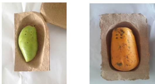
Figure 15. Packaging made from heliconia pulp mixed with galangal stem extract water
