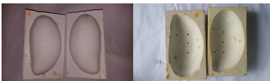
Figure 2. Pores at the bottom side of the lower mold. (left) The upper mold (right)
