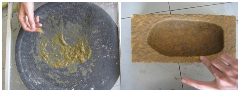
Figure 6. Pulp being prepared. (left) Tapping pulp onto the lower mold. (right)
