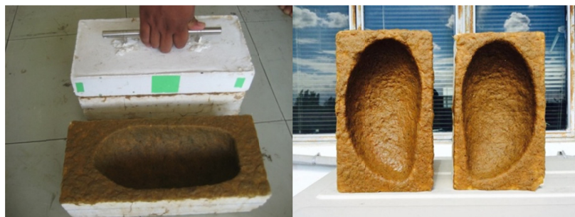
Figure 7. Press the upper mold onto the lower mold with tapped pulp. (left) The mold was sun dried (right)
