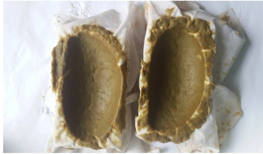
Figure 4. Produce packaging by pouring pulp
