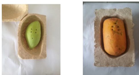
Figure 14. Packaging made from heliconia pulp mixed with kaffir lime leaves extract water
