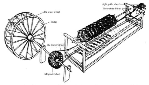
Figure 1. A reconstruction of the water-propelled large spinning wheel based on the data provided by Wang Zhen in his "Nong Shu"
