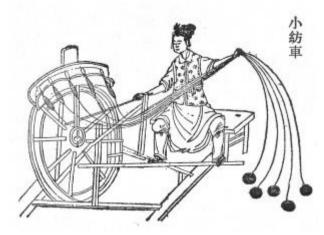
Figure 6. An illustration from "Nong Shu", depicting the spinnig wheel specially designed for twisting ramie strands
