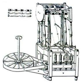
Figure 4. The Arkwright's water-propelled spinning frame
