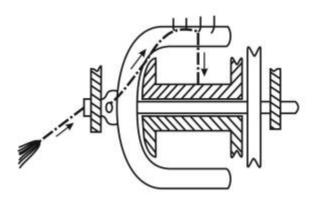
Figure 5. The construction of Saxony spinning wheel
