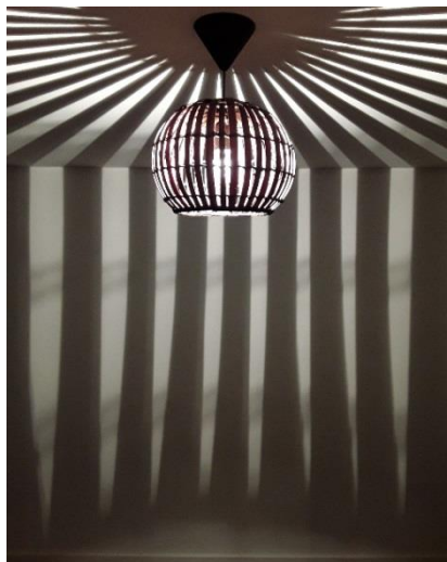
Figure 1. The light source consists of a spherical structure with a diameter of 29.5 cm, sectioned at the bottom. It is composed of 42 vertical bands, each with an average width of 1.26 cm, which create 42 slits with an average width of 0.95 cm at mid-height. The structure can accommodate a bulb positioned at its center, featuring either one or two vertical filaments
