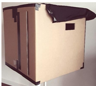
Figure 2. The box used has approximate dimensions of 60 cm × 60 cm × 60 cm. A box with slightly greater depth between the slit and the screen and/or increased height can also be used. However, it is preferable to limit the width to ensure that the horizontal movement of the fringes on the screen remains minimal throughout. On one side of the box, there is a tall vertical slit, and positioned in front of it is a white screen
