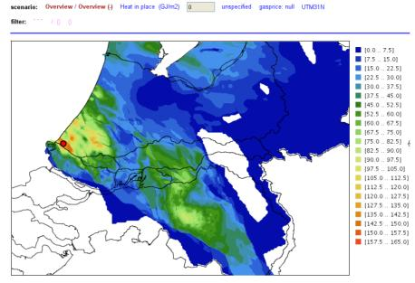
Figure 1. Heat distribution of the potential warm geothermal energy
