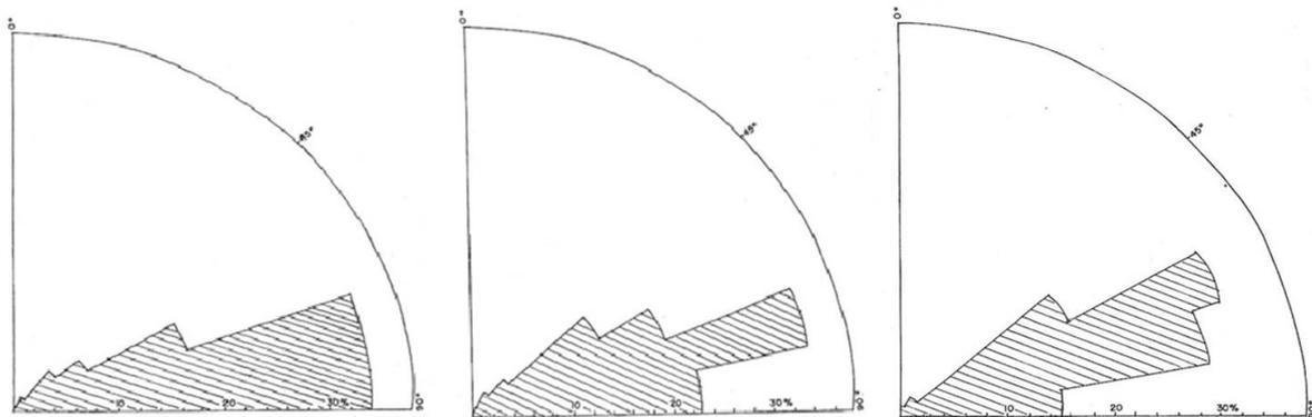
Figure 13. Showing joint dips in Oban Massif: A, in schist (373 data points); B, in gneisses (230 data points); C, in granodiorite (191 data points)
