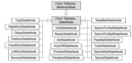
Figure 4. Control states defined as sub-classes of Tekkotsu's StateNode class
